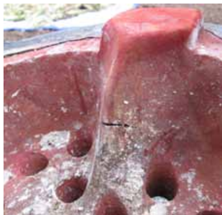
On the left, crack on the ceramic wall of the combustion chamber. In the center, a broken grate of the combustion chamber. On the right, displacement between the ceramic inlet and the sealing.
