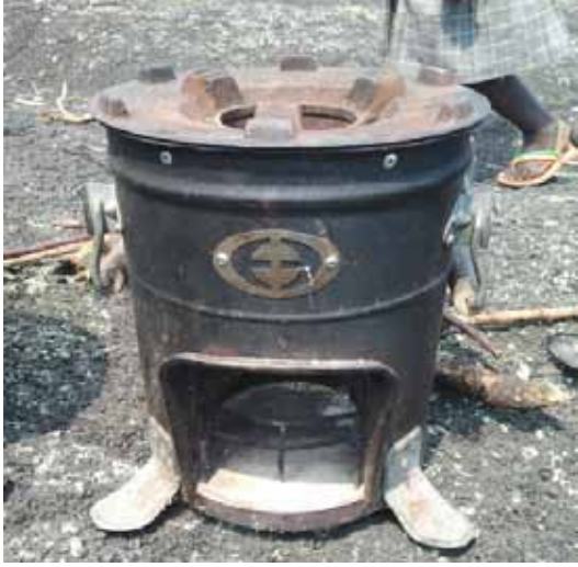
Envirofit M-5000 fuel-efficient firewood stove after 10 months of use in Nzulo camp
