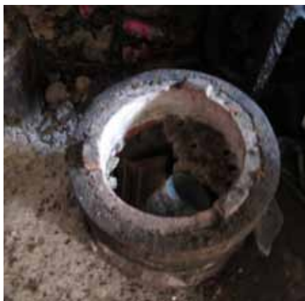
On the left, crack on the ceramic wall of the combustion chamber. In the center, a broken grate of the combustion chamber. On the right, displacement between the ceramic inlet and the sealing.
