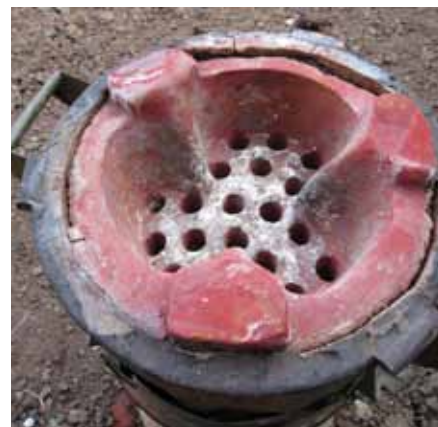
On the left, crack on the ceramic wall of the combustion chamber. In the center, a broken grate of the combustion chamber. On the right, displacement between the ceramic inlet and the sealing.
